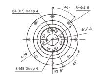
Input Shaft Diameter  $\leq \phi 8$  (in mm)
