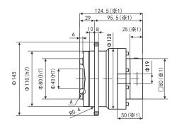
Input Shaft Diameter  $\leqslant \varphi \, 28 \,$  (in mm)
