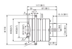
Input Shaft Diameter  $\leq \phi 14$  (in mm)
