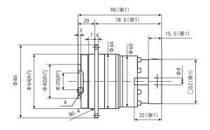
Input Shaft Diameter  $\leq \phi 14$  (in mm)
