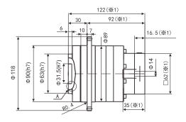
Input Shaft Diameter  $\leq \phi$  19 (in mm)
