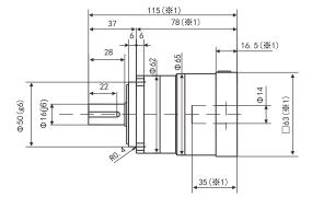
Input Shaft Diameter  $\leq \phi$  19 (in mm)
