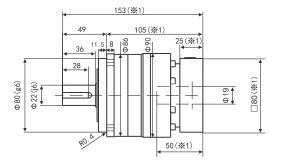
Input Shaft Diameter  $\leq \phi 28$  (in mm)
