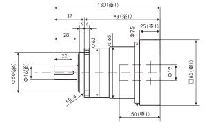
Output Shaft Type (in mm)
