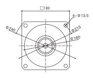
Output Shaft Type (in mm)
