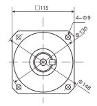
Output Shaft Type (in mm)
