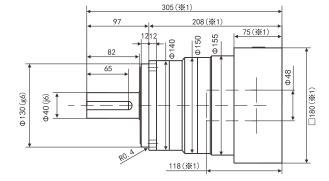
Output Shaft Type (in mm)
