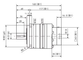
Input Shaft Diameter  $\leq \phi$  19 (in mm)
