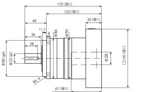
Input Shaft Diameter  $\leqslant \Phi$  8 (in mm)
