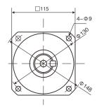
Output Shaft Type (in mm)
