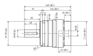
Input Shaft Diameter  $\leq \phi$  38 (in mm)
