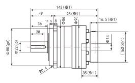
Input Shaft Diameter  $\leq \phi$  19 (in mm)
